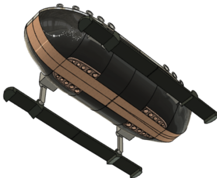
Fig. 5. Underneath the rover, showing the keel line and channels for gas to move through
